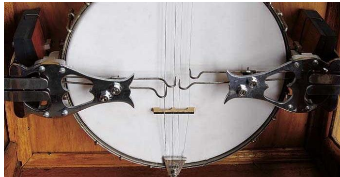
Figure 12: Boston version of the Encore. Left: note yet a third shape of the shield surrounding the banjo neck; Right: Picker mechanism unique to the Boston machine.
