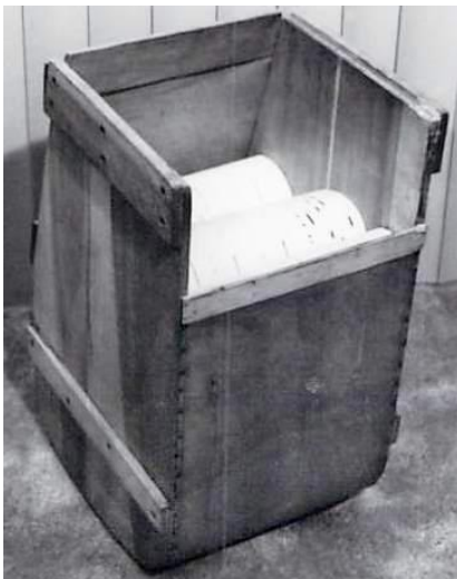
Figure 15. Basket holding an Encore endless roll. These were easily slid out to change rolls without rewinding. Is this the first cassette?
