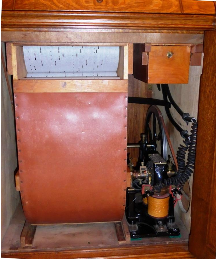
Figure 20: Early Crocker-Wheeler motor powering an Encore Banjo. The endless-music roll in its basket is visible on the left and wooden coin box above.
